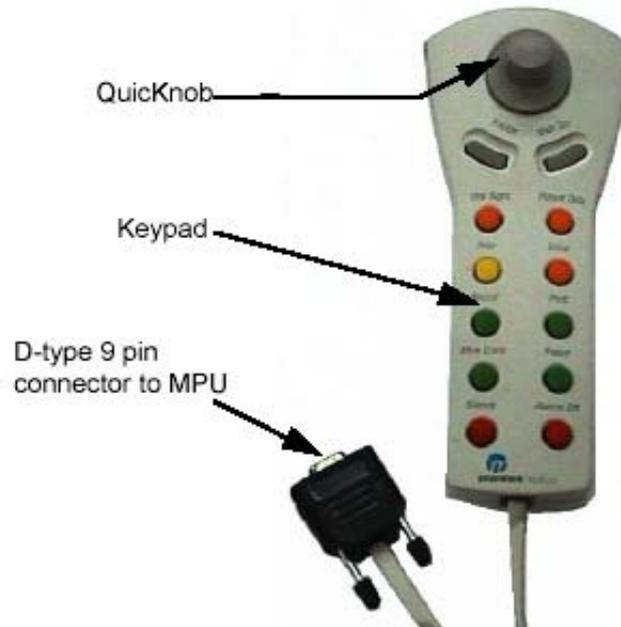
Figure 1-3: The VitaLogik Remote Keypad
