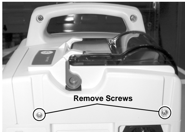
Figure 7-1: Remove Screws from Printer Assembly
